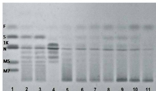
Fig. 4. Chromatoplate of standards, chicory and Agave FOS. Line 1: standards (F, fructose Rf 0.38-0.47; S, sucrose Rf 0.36-0.39; 1-K, 1-kestose Rf 0.28-0.29; N, nystose Rf 0.25-0.27; M5, maltopentaose Rf 0.14-0.17; M7, maltoheptaose Rf 0.09-0.10), 2: Chicory FOS Sigma, 3: Orafiti GR, 4: P95 Orafiti, 5: CIATEJ Agave FOS, 6 to 11 commercial Agave fructans, 6: Fag, 7: Fan, 8: Faa, 9: Fac, 10: Fap, 11: Fai.
